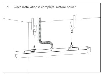
The installation must be carried out by a qualified electrician.
